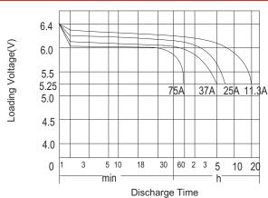
(Note) The above characteristics data are average values obtained within three charge/discharge cycles not the mimimum values.
